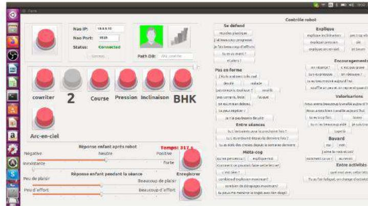
Figure 6.1: WoZ Interface. On the left side, the therapist can connect to the robot (top), choose the activity to engage the child in (centre), and annotate the child's responses to the robot's behaviour (bottom). On the right side, buttons to trigger various robot behaviours.
